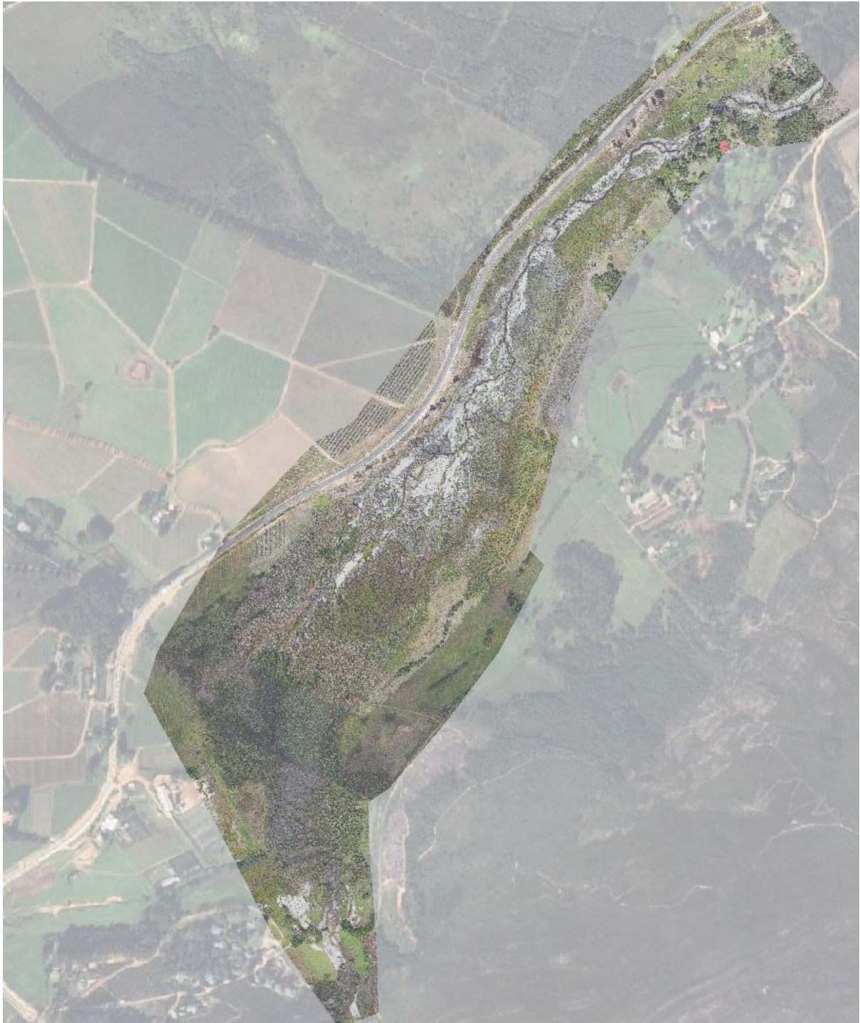
Figure 19 The orthophoto produced with drone-based photogrammetry on a Google Earth background. This shows the extent of the area surveyed for the construction of the hydraulic simulation models.
