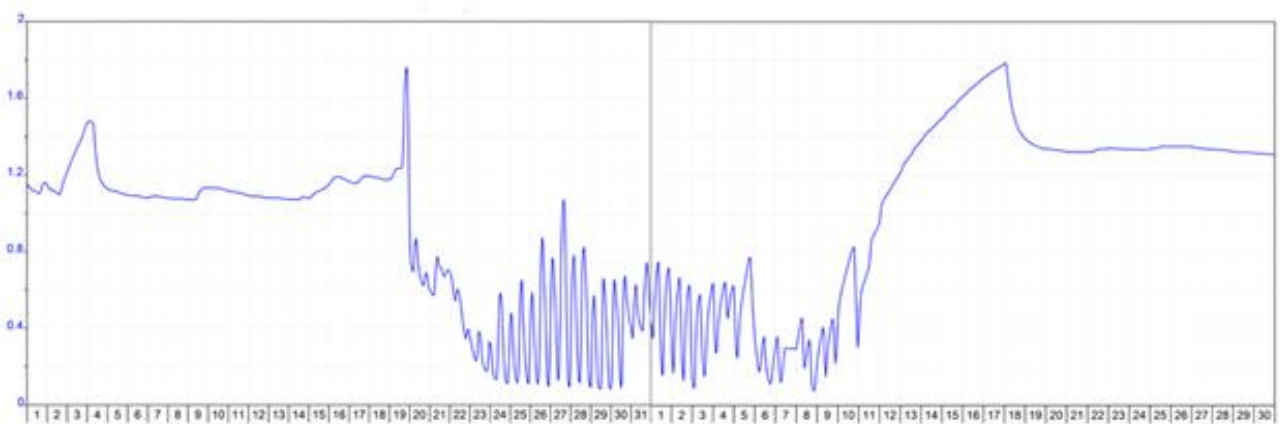
Figure 3-4. Data from the Onrus Lagoon water level gauge plotted for one-hour intervals for the period 1 October to 30 November 2012. The lagoon breached naturally on 19 October 2012 following heavy rainfalls. (Source: DWS).
