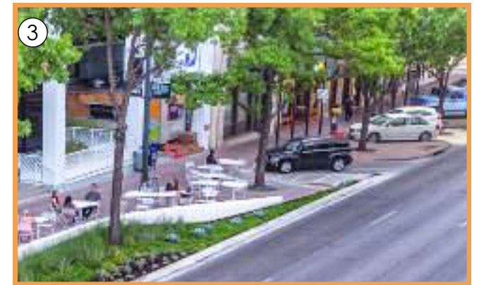
3. Intermittent parallel parking and widened, landscaped sidewalk ensures both cars & people are accommodated.
