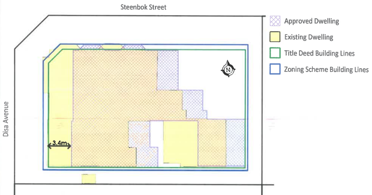
Figure 2: Approved versus As-Built Position of Structures
