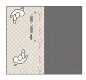
Bollards should be placed at a regular intervals and in a straight line.
