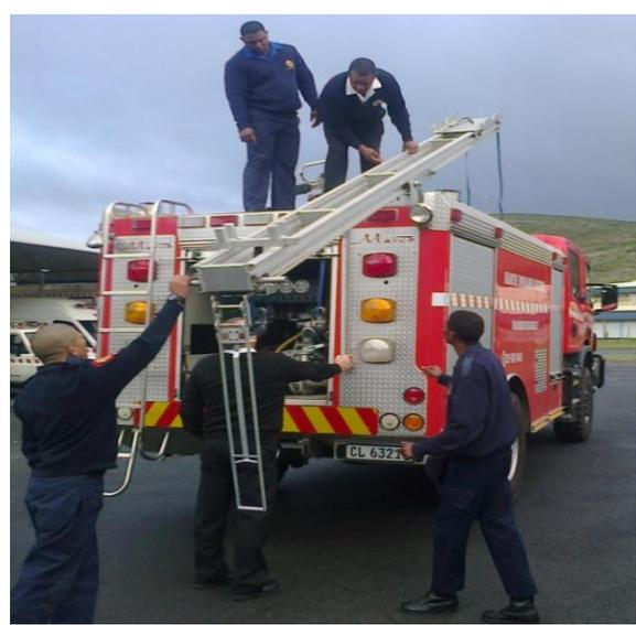
LADDER GANTRY TO REMOVE THE LADDER FROM THE ROOF OF APPLIANCES TO THE GROUND. (Par 2.17)
