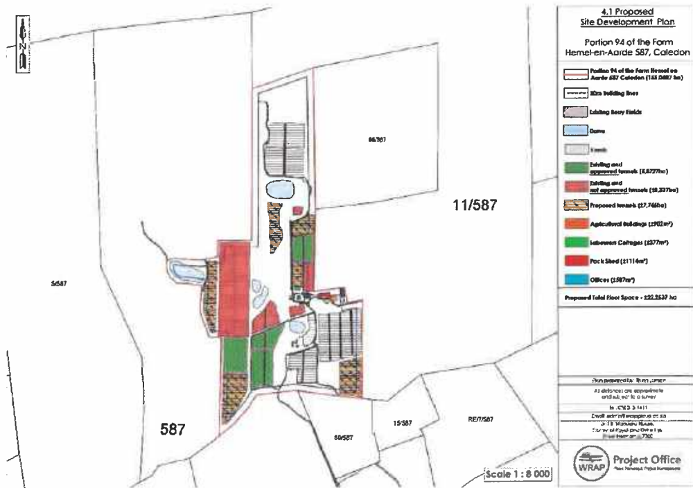
Figure 4: Proposed Site Development Plan: Illustrating the parameters and extent of new and existing horticulture tunnels and required set back lines. Source: WRAP Project Office
