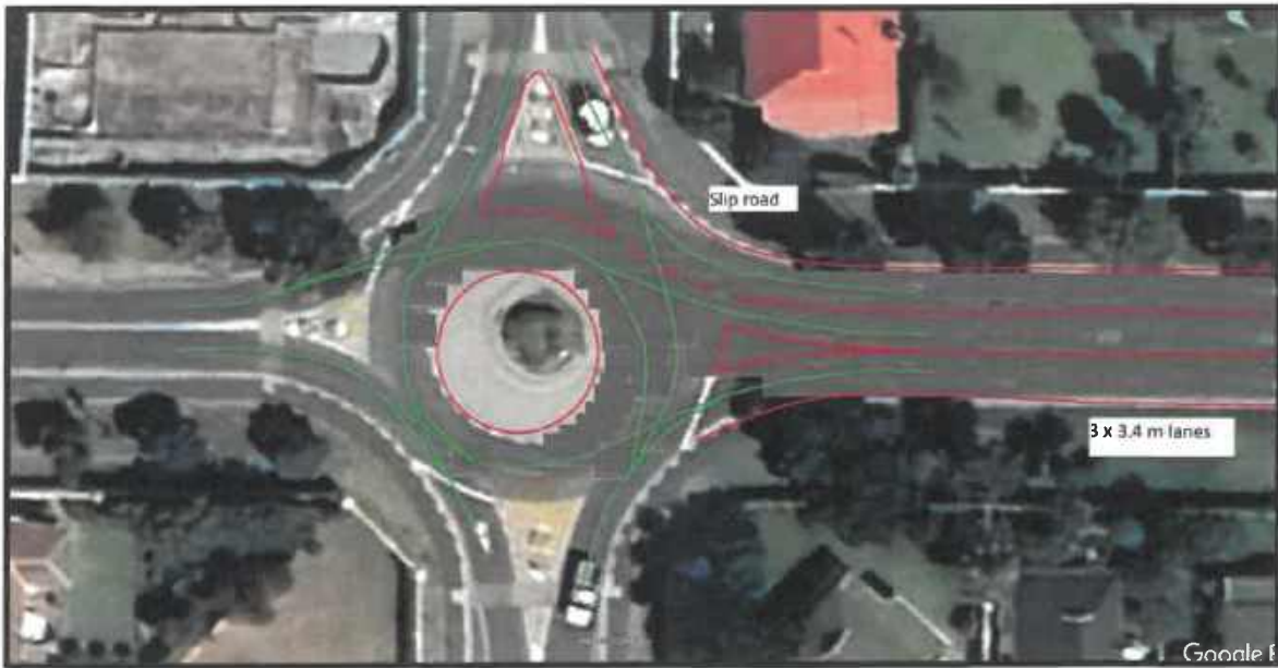
Figure 4: Conceptual layout of slip road at roundabout
