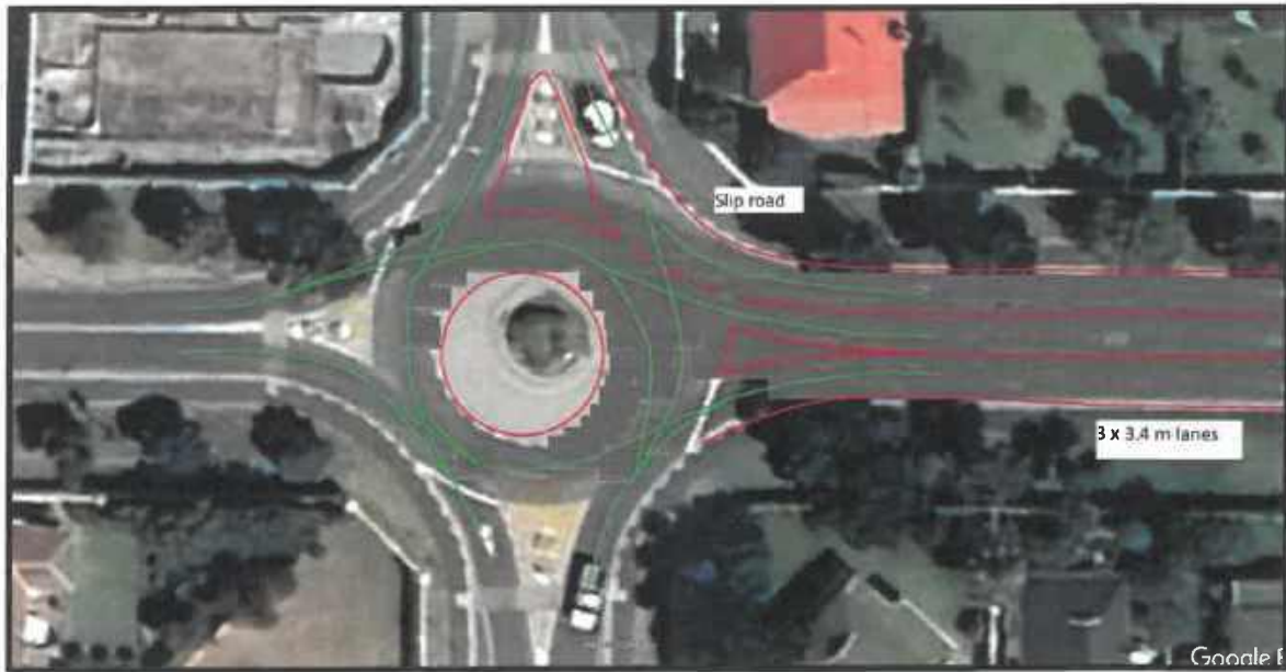
Figure 4: Conceptual layout of slip road at roundabout
