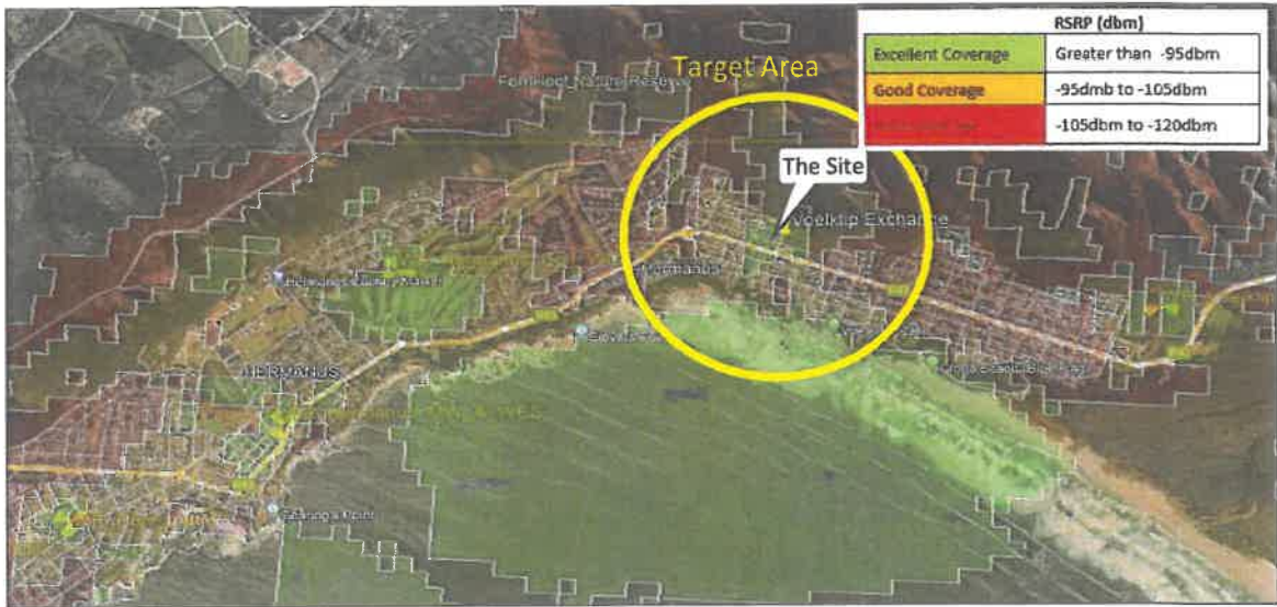
Figure 7 – Telkom After Coverage Prediction @15m at Erf 6679 Hermanus
